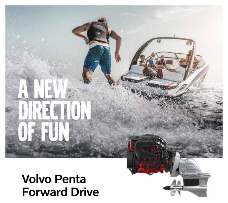
Volvo Penta Forward Drive – the new standard for getting the most fun out of your boat. Twin counter-rotating, forward-facing propellers pull the boat rather than push it for higher top speeds, faster acceleration and superior maneuverability. And maybe a quickened pulse. The result is a propulsion system capable of big wakes, smooth cruises and everything in between.
