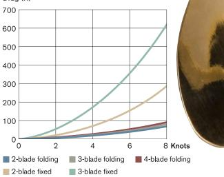
This graph shows how rapidly the propeller drag increases with higher speed. At 8 knots for example, a 3-blade fixed propeller produces more than six times the drag of a 3-blade folding propeller.
